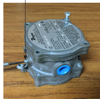
Air proving pressure switch adjustment
