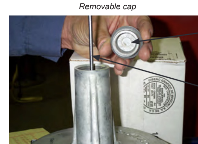
Use screwdriver to adjust regulator
