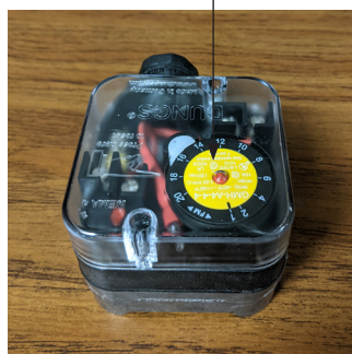
Air proving pressure switch adjustment
