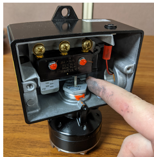
Gas or Oil pressure switch adjustment – Type B
