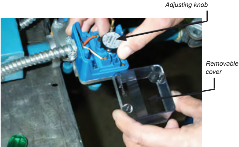
Gas pressure switch adjustment – Type A
