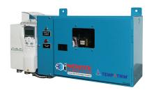
Webster Combustion's patented TEMP-A-TRIM air density trim system senses combustion air temperature and automatically varies the fan speed to create a constant mass air flow for combustion. By maintaining optimum fuel/air ratios, the UL-approved TEMP-A-TRIM ensures maximum burner efficiency.
