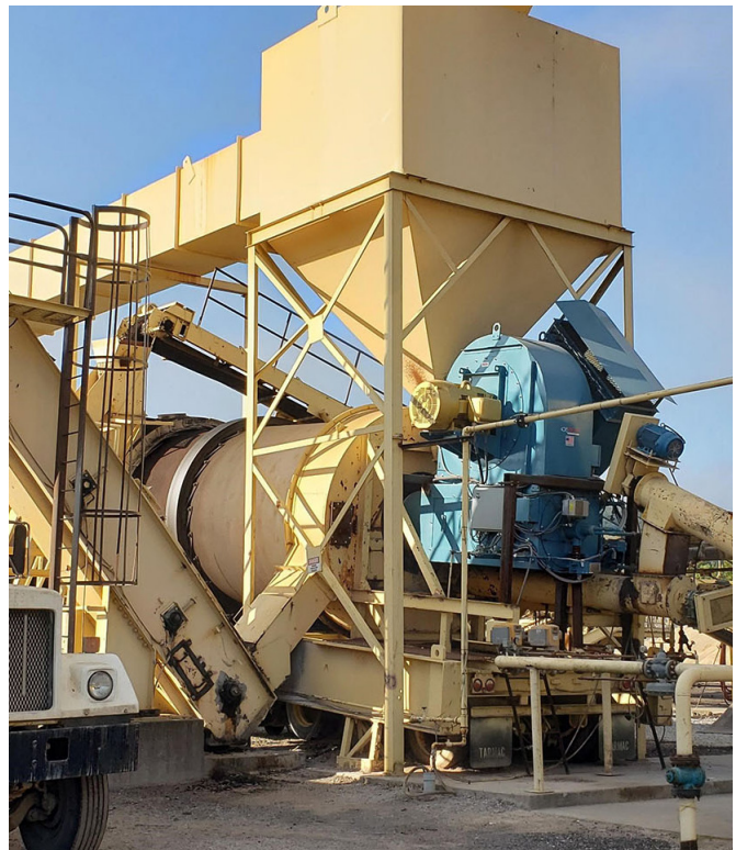
Before the burner retrofit (left), and after (right), showing the new Webster Combustion model HDRA-RF, operating as a total air-fired burner at 125,000,000 BTU to dry 400 tph of aggregate.
