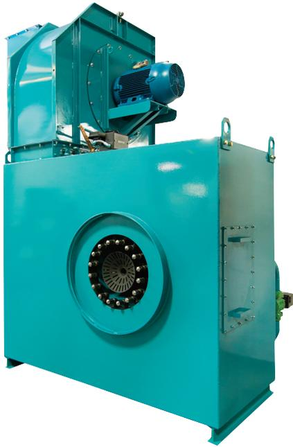
Webster's FDR(X) Forced Draft Register burner is a highly efficient combustion system that combines a windbox, air register, ignition assembly, fuel train, flame safety control, combustion control, FGR (Flue Gas Recirculation) system, and a forced draft blower, all assembled into **one complete packaged unit**.
