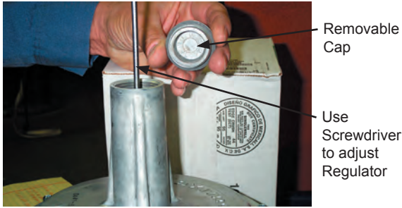
Figure E – 9 Main Gas Pressure Regulator Adjustment
