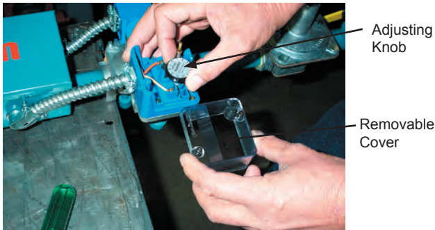
Figure E – 10 Gas Pressure Switch Adjustment
