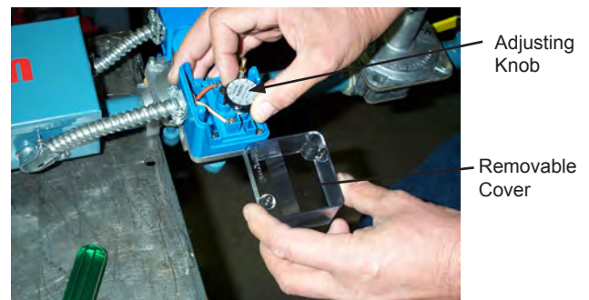
Figure E – 8 Gas Pressure Switch Adjustment
