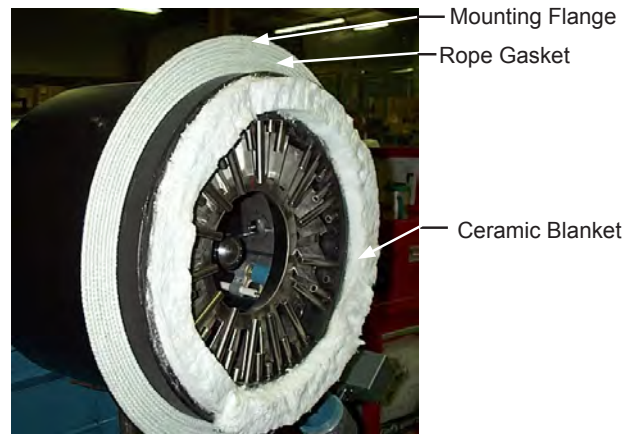
Figure B-13 Gas Manifold
