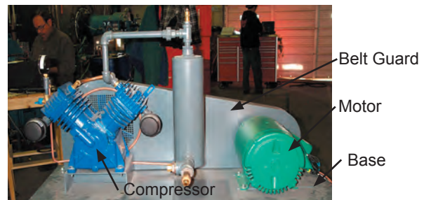
Figure B-21 Small Air Compressor
