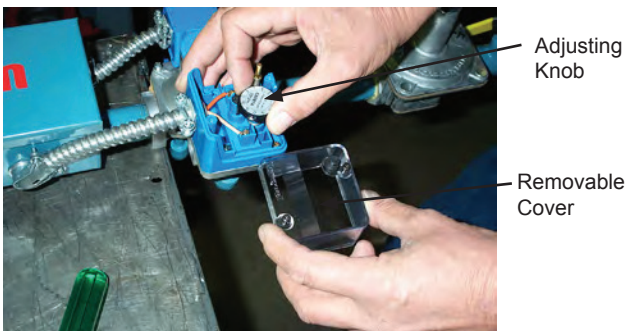
Figure E – 10 Gas Pressure Switch Adjustment
