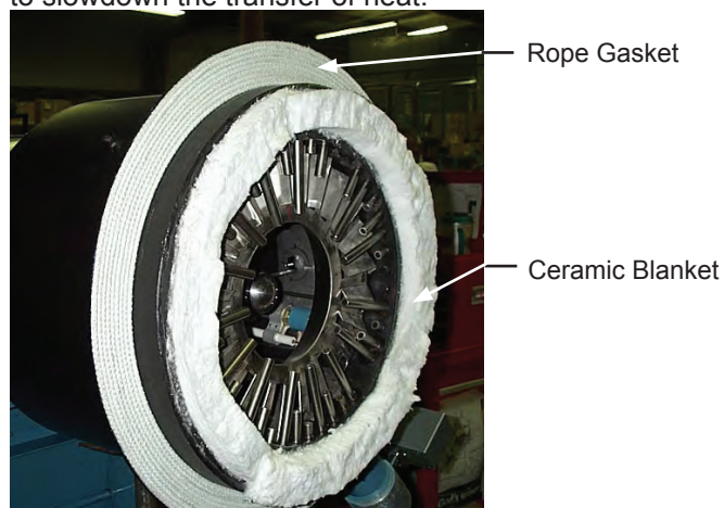
Figure B-14 Gas Manifold
